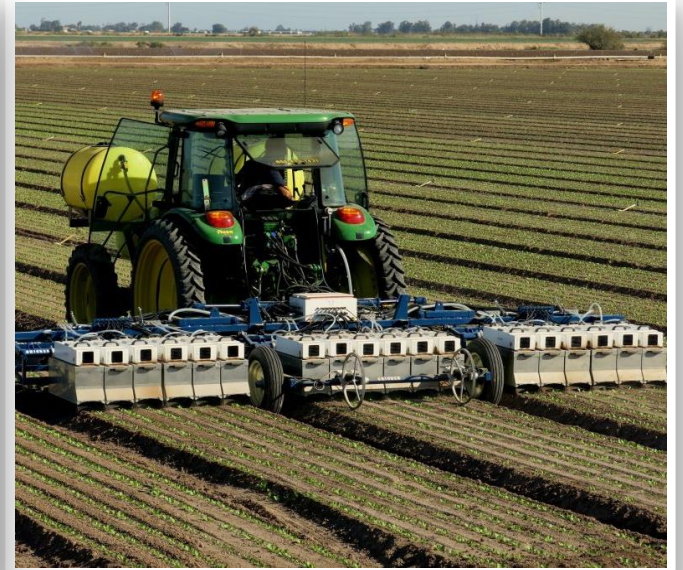
Separating weeds as it harvests, reduces chemical usage by 90%
