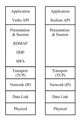
Figure 1. iWarp and TCP Protocol Stacks.
