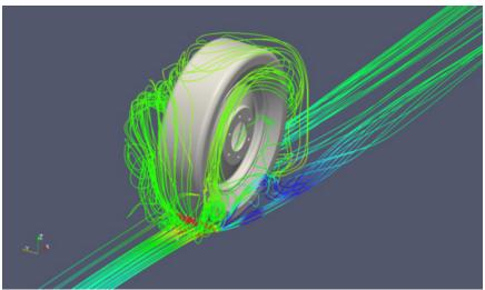
In a simulation run at the Ohio Supercomputer Center, an isolated view of a wheel on the Buckeye Bullet illustrates airflow within the wheel well with the vehicle traveling at 300 mph
