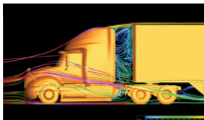
A truck aerodynamics (CFD) simulation Courtesy of BMI/SmartTrucks
